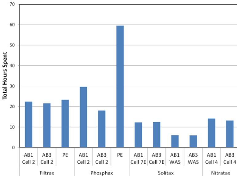
**Figure 7.** Operation and maintenance hours for continuous monitoring devices tested during Durham instrumentation pilot [11]
