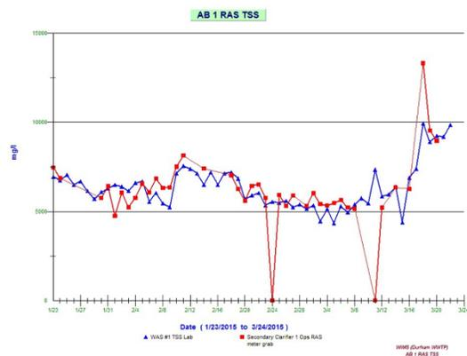
**Figure 6.** Continuous TSS data (red) compared to lab results (blue) in return activated sludge from aeration basin1 at Durham [11]
