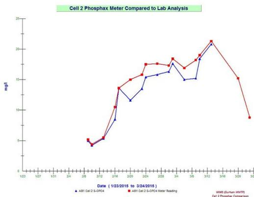
**Figure 5.** Continuous OP data (red) compared to lab results (blue) in Durham cell 2 [11]
